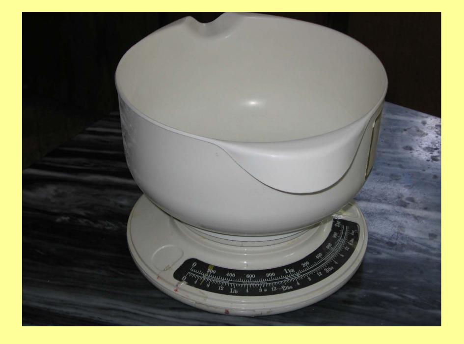
This kitchen scale is calibrated in ounces and grams. Our recipe is measured in metric weight, rather than volume, as weight provides greatest accuracy (your cup of flour might not weigh the same as my cup of flour). Also, metric measurement (because it's based on parts of 10) is easy to calculate when you want to multiply or divide to increase or decrease a recipe.
